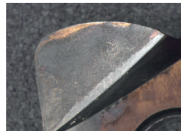
Flank and Rake wear after 45 min
