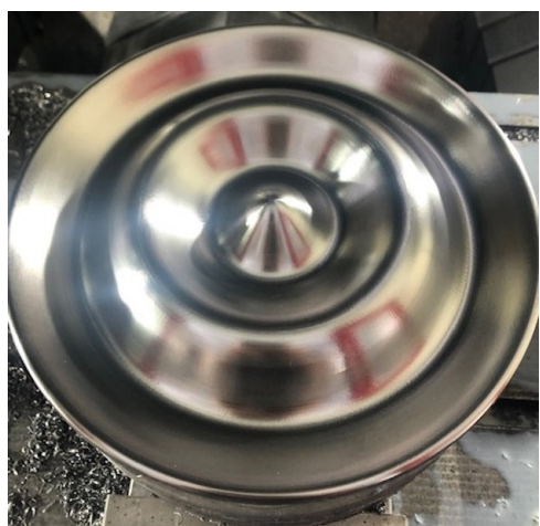
Surface finishing with more challenging cutting conditions
