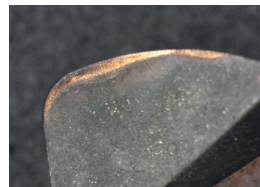
Flank and Rake wear after 67 min
