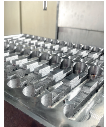
Interrupted Pocket milling operation
