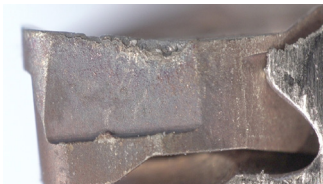
Tool wear after 85 minutes of machining
