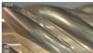
Test 1: Tool wear after 8 hours and 30 minutes of machining
