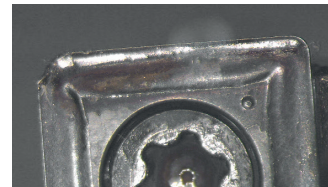
Tool wear after 16 hours of machining
