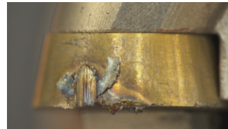
Flank wear after 114,4 cm 3 of material removed
